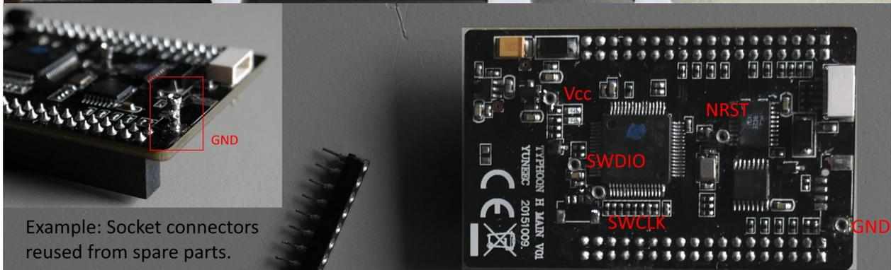
Example: Socket connectors reused from spare parts.
