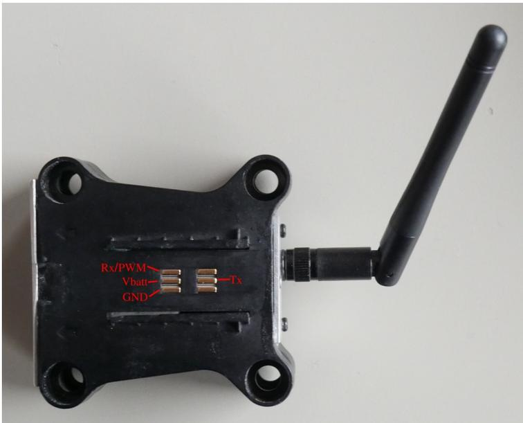
The antenna connector on ESP8266 MCU module is the same as used for the ST16 antennas (and many others). Please keep in mind you cannot use the 5GHz mushroom antenna for the MCU board. It uses **2.4GHz** WiFi band. You need an antenna for 2.4GHz if you want to have a better one.
